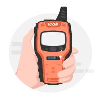
[Transponder detection]: press the power button for 1 second [Frequency test]: press and hold the power button for 2 seconds
