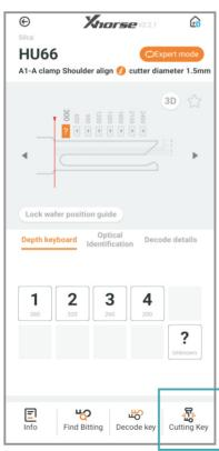
4) According to the prompts on the page, confirm the clamp type and adjust the clamp position. Enter the known key bit and click "Cutting key" after confirming that it is correct.
