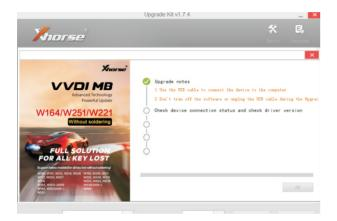
5) The upgrade kit automatically writes the file. It takes a few minutes. After the upgrade is completed, click "Confirm" to complete the upgrade.
