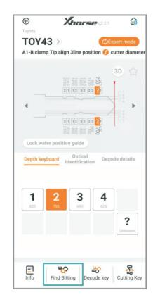
4) Enter the known key bit, if the key bit is not clear, directly enter "?" and click "Find Bitting" after input. It can be processed according to the key bit which calculated by the system.
