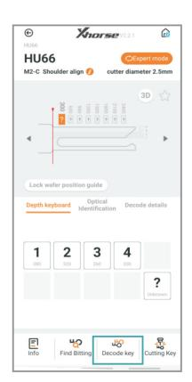
1) Enter the key to be operated interface, and click "Decode key".
