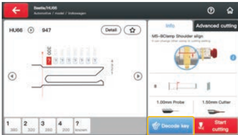
6) After setting the key blank according to the diagram on the right and click "Decode key". (The clamp picture on the Info can be enlarged to see more clearly.)
