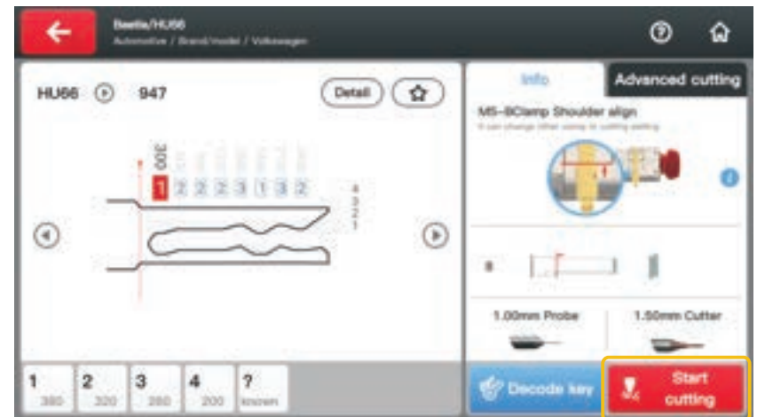
5) Install the key blank according to the diagram on the right, enter the key code and click the "Start cutting" button.
