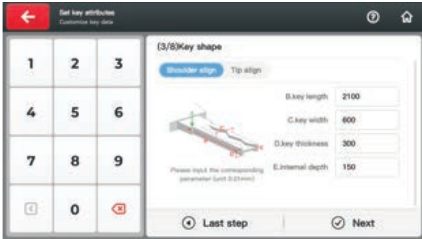
4) Select shoulder align or tip align and enter the corresponding parameters of the key.
